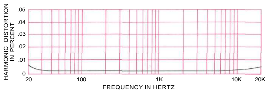
MONITOR AMPLIFIER HARMONIC DISTORTION 20 WATTS OUTPUT PER CHANNEL, 8 OHMS
